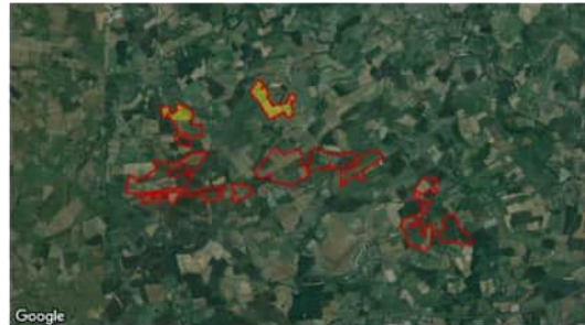
Observer Location Sun azimuth range is 79° - 91° (yellow)
