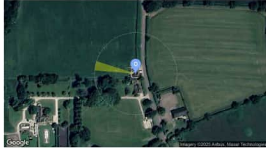
Observer Location Sun azimuth range is 274.7° - 287.9° (yellow)
