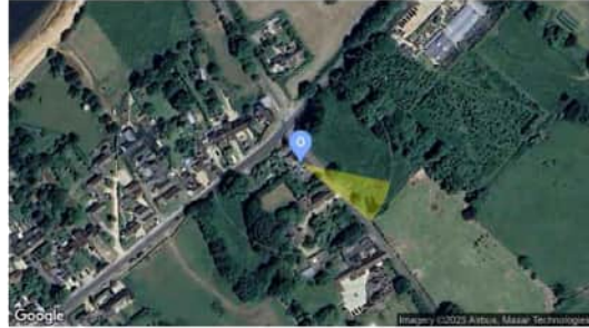
Observer Location Sun azimuth range is 101.9° - 129.6° (yellow)
