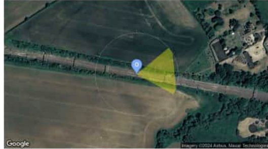
Observer Location Sun azimuth range is 50° - 118.7° (yellow)
