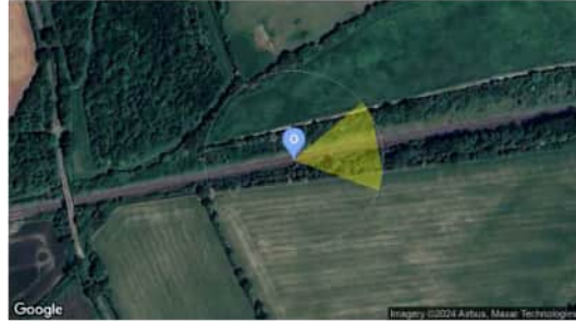
Observer Location Sun azimuth range is 49.3° - 109.8° (yellow)
