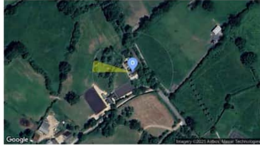
Observer Location Sun azimuth range is 270.3° - 287.3° (yellow)
