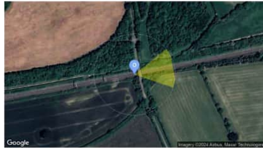
Observer Location Sun azimuth range is 51° - 108.7° (yellow)
