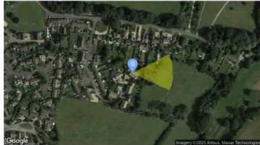
Observer Location Sun azimuth range is 61.8° - 114.9° (yellow)
