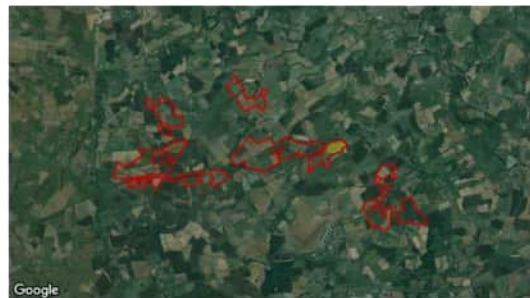
Observer Location Sun azimuth range is 264.9° - 279.2° (yellow)
