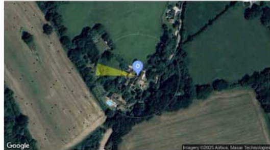
Observer Location Sun azimuth range is 270.5° - 287.3° (yellow)
