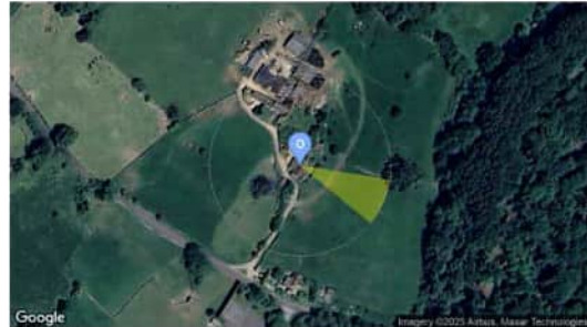
Observer Location Sun azimuth range is 99° - 129.5° (yellow)
