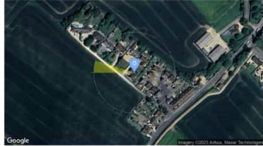
Observer Location Sun azimuth range is 269.8° - 287.4° (yellow)
