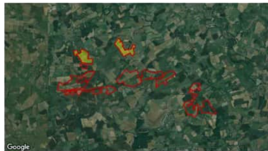
Observer Location Sun azimuth range is 270.6° - 285° (yellow)
