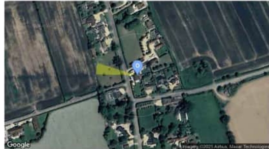
Observer Location Sun azimuth range is 271.3° - 287.3° (yellow)
