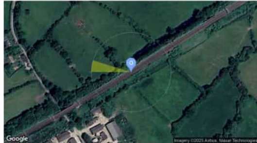
Observer Location Sun azimuth range is 270.3° - 287.3° (yellow)
