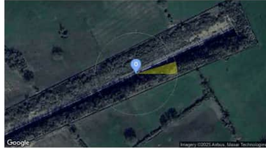
Observer Location Sun azimuth range is 72.8° - 90.2° (yellow)
