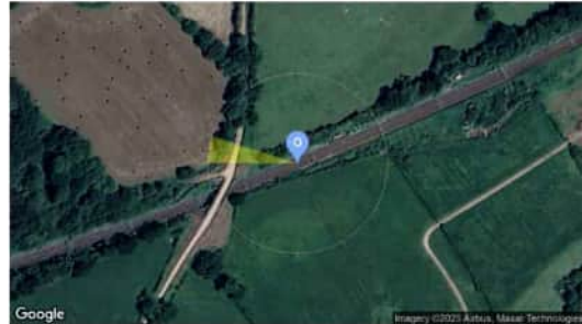
Observer Location Sun azimuth range is 270.4° - 287.9° (yellow)
